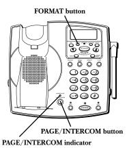
Press the PAGE/INTERCOM on the base or INT button on the handset where the outside call is in progress.
